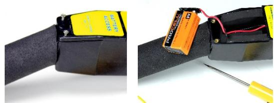
The 9v battery is located inside the battery access area and is attached to a battery terminal connector. The battery connector can be removed by firmly grasping the battery with one hand and the connector with the other and pulling apart. Do not use a screwdriver or any prybar made of a conductive material to separate the battery from the connector.
