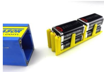
Figure 8 – slide battery sled back into case, closed end first
