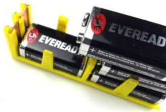
Figure 15 – all batteries must be installed the same way
