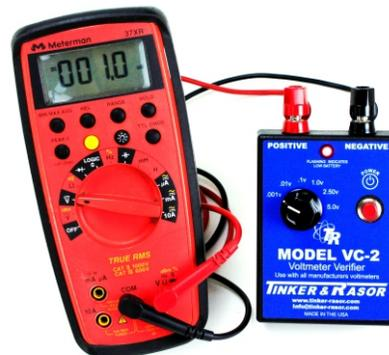
The VC-2 works with any manufacturers voltmeter to verify accuracy.
