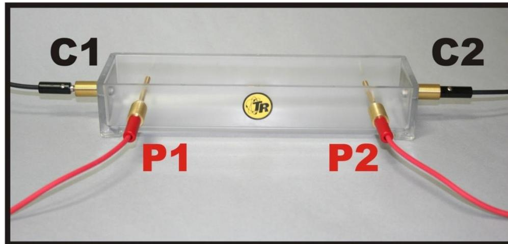
Model SB-1 multiplier for 4 Pin measurements is 1.349.
