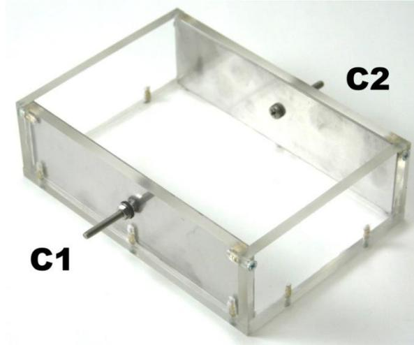
When using this soilbox, the pin selection switch should be set to “2 PIN” method. As shown below. Model SB-2 multiplier per AASHTO T-288 is 6.67 cm
