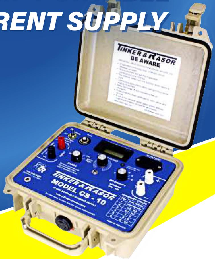
*The CS-10 portable current supply is an ideal DC current source for many cathodic protection corrosion maintenance tests. Commonly used for determining current requirements for cathodic protection or impressing current on an underground structure for assisting in locating electrical contacts with foreign systems such as underground utilities.*
